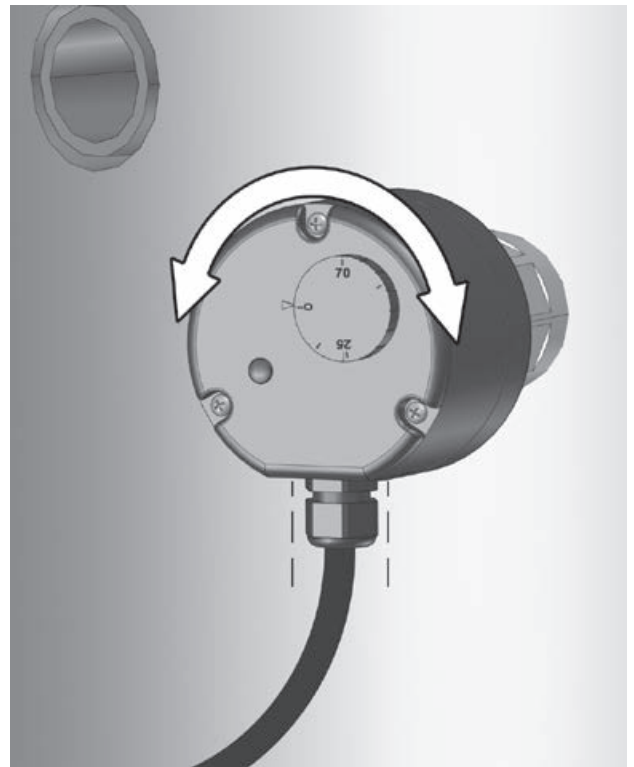
Illustration 13: Align screwed cable gland
