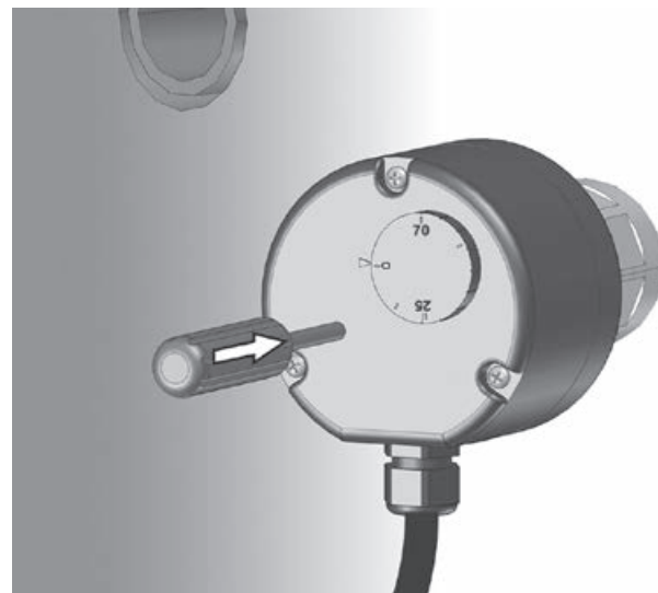
Illustration 17: Fuse resetting with the help of a screwdriver
